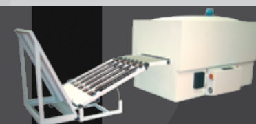
Quartz Post-bake Oven with a Plate Stacker at the end.
